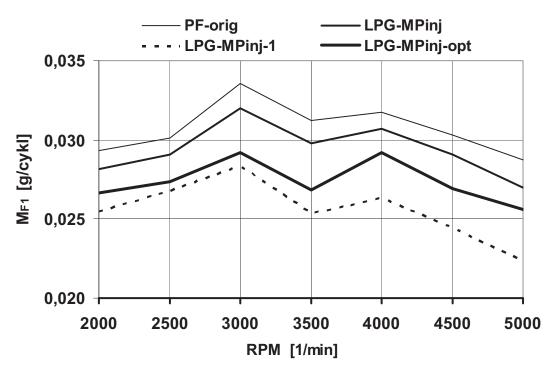
Fig. 10. The injected fuel quantities for full load conditions at running on PF and on LPG for different variants of the experimental engine they reflect the right functional coupling original ECU of PF engine on ECU Vialle fuel system for injection of the liquid LPG
