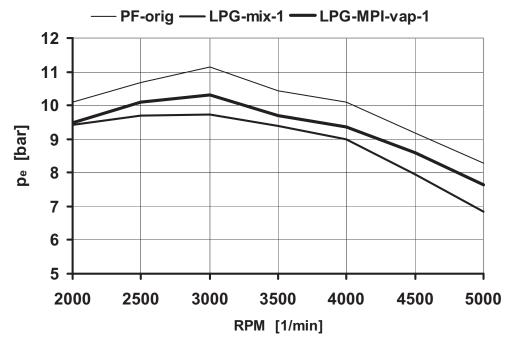
*Fig. 3. Disposable values of the BMEP throughout the engine working cycle for full load at running on PF and on LPG (variant with the mixture forming by mixer and by multipoint injection of evaporated LPG)*
