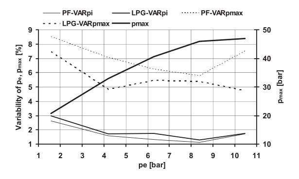
Fig. 8. Combustion peak pressures on load characteristic at  $RPM = 3000 \ 1/min$  they have at engine running on PF and on LPG virtually like the same values, the parameters of the intercycles variability for PF and LPG they are for  $p_i$  as well comparable, the engine running on LPG has a somewhat lower values of intercycles variability for  $p_{max}$  (by using statistical processing of the set 150 sequential following cycles)
