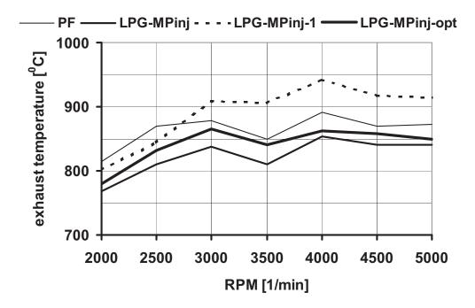
Fig. 5. The courses of exhaust gas temperature in full load conditions for experimental SI engine running on PF with original ECU for regulation of the mixtures richness and for running on LPG with different setting of the air/fuel ratio governing
