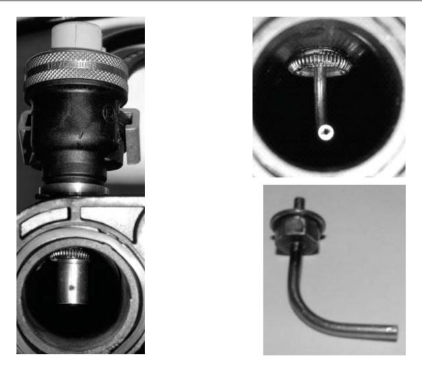
*Fig. 1. The LPG injector placed on the inlet engine manifold and chambered nozzle in the inlet manifold (left), pipe's nozzle in the intake manifold and the view on the type of pipe's nozzle (right)*
