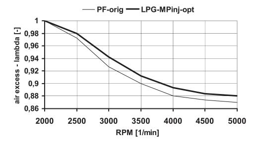
Fig. 6. The optimized governing of the mixture richness for full load conditions of the experimental SI engine with injection liquid of LPG to the intake manifold in face of intake port at cylinder head
