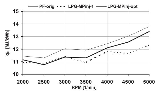
Fig. 11. Specific consumption of the heat on full load speed characteristic for different variants of experimental engine
