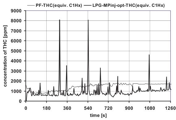
Fig.12. The course of the THC concentration from metering on experimental SI engine with injection of liquid LPG (fuel system VIALLE) at full load speed characteristic (with the electronic data acquisition from analyzer at 5s step) at comparison with the course of the THC concentration from metering on engine PF running
