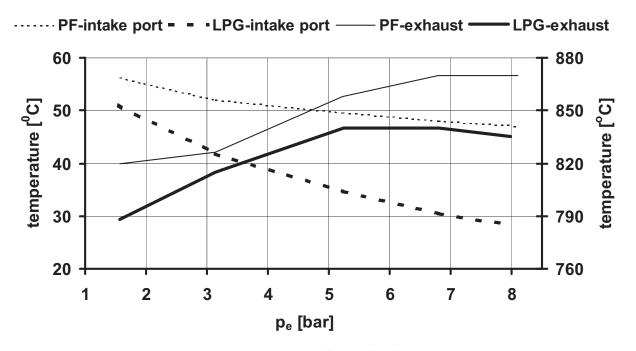
Fig. 4. Fresh mixture temperature in intake port at cylinder head and exhaust gas temperature at 5000 rpm (the temperature in the intake port is determined as arithmetic mean of 16-18 recorded temperatures for each measurement point, the exhaust gas temperature there is calculated as arithmetic mean from several points at the end of each measurement mode)
