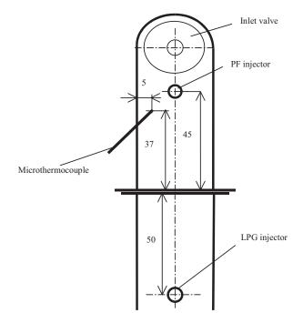
*Fig. 2. The scheme of microthermocouple in the intake port in cylinder head for metering air (mixture) temperature before the intake valve. The scheme of dimension location for measuring temperature in the intake port of the engine (dimensions shown are reached at extended central axis of the port)*
