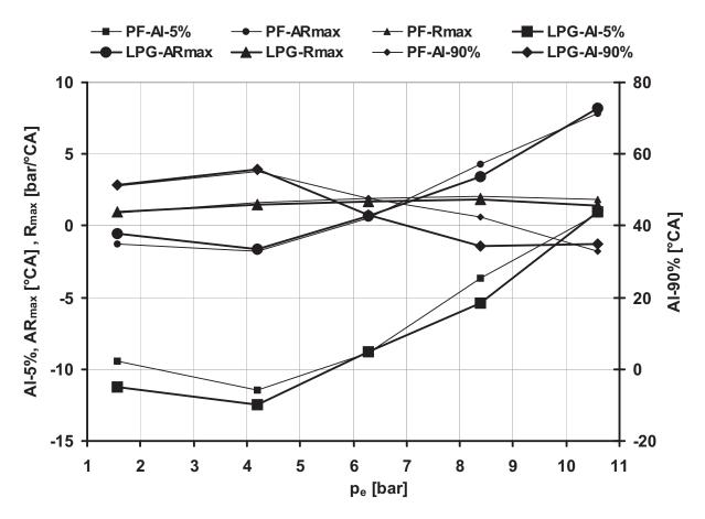
Fig. 9. The parameters of the course of mixture combustion at cylinder at running on PF and on LPG on load characteristic at RPM = 3000 1/min
